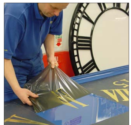
Removing mask after applying gold leaf to a replica dial for a stately home.
