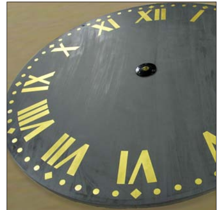
After: original perfectly replicated in GRP.
