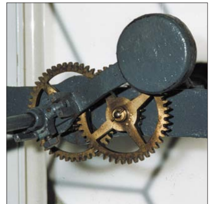
Dialworks and hand counterbalances behind an exterior dial.
